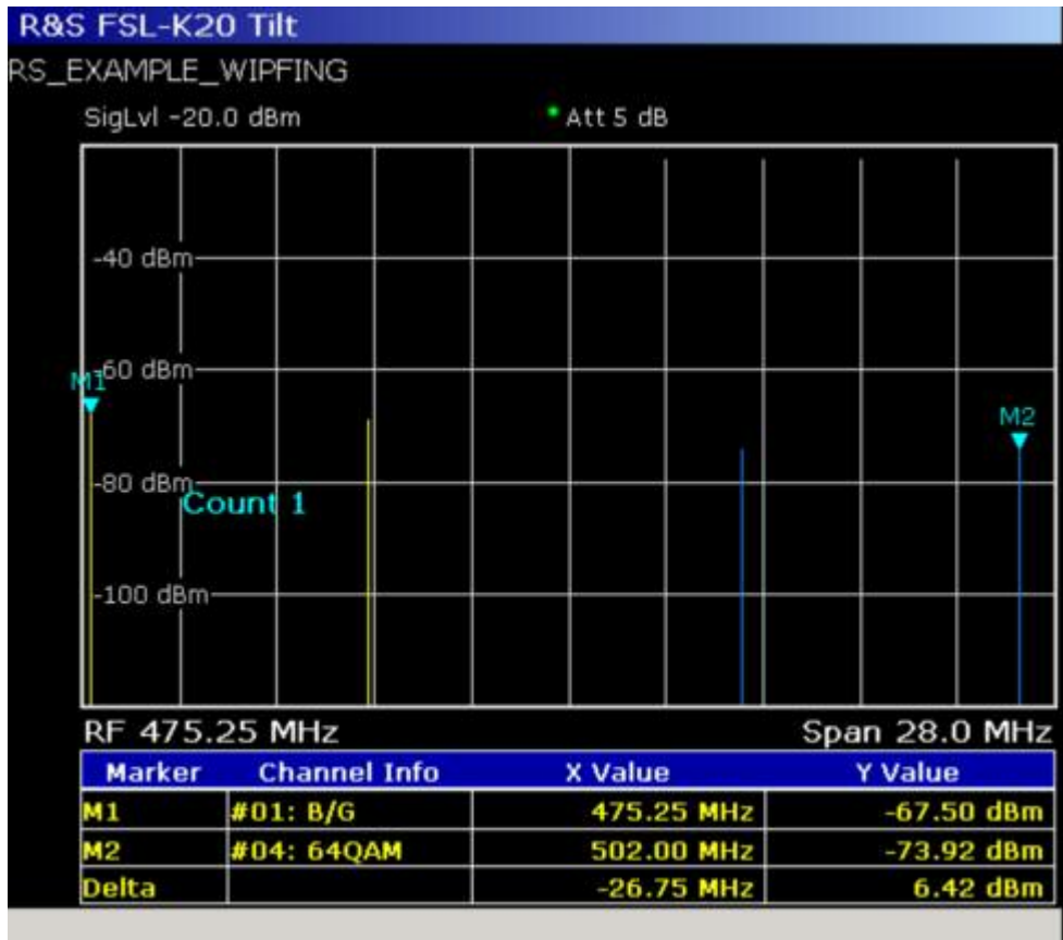
Fig. 2-72 Tilt measurement using a Channel Table. No input signal!
