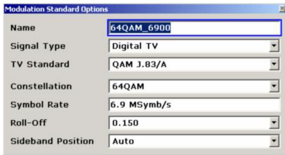
Fig. 2–67 Digital TV modulation standard 64QAM_6900
